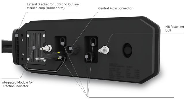
$4x\ 2\mbox{-pin}$  AMP superseal connectors for additional lighting:
